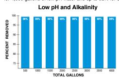
Test data generated by certified national laboratory using the protocol described in NSF Standard 53 using a flow rate of 0.75 gpm and an average feed of 150 ppb lead. Water's pH was 6.5 and alkalinity 10-30 ppm as CaCO<sub>3</sub>.
