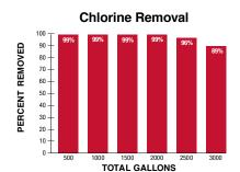
Test data generated by independent laboratory at 1 gpm using test procedures described in NSF Standard 42. Average chlorine feed at 2 ppm.
