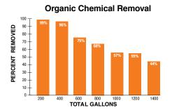
Test data generated by independent laboratory at gpm using test procedures described in NSF Standard 53. TCE used as test contaminate at average feed of 300 ppb.
