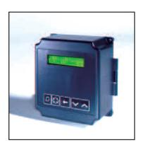
The 3214NXT Demand Flow Network Controller is available to configure with all commercial Fleck® 2750, 2850, 2900, 3150, and 3900 Control Valves. This demand flow system can be programmed to bring multiple units to the service position and back to standby based on system demand flow. The 3214NXT Demand Flow Network Controller uses on-board communication capabilities to link multiple valves via standard CAT3, CAT5, or better communication cables.
